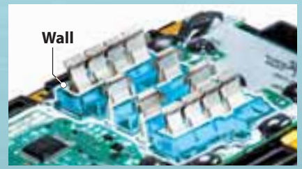
Terminal short-circuit prevention structure The protection wall is provided between terminals against water and dust.
