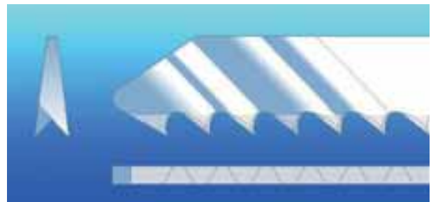
Ground and taper ground teeth
