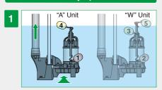
The next time the water level rises. Float #1 on the "A" unit is activated but the unit does not start until Float #4 is activated
