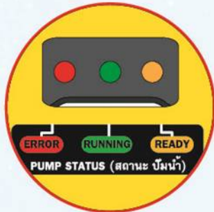
LED Status (On terminal box)
