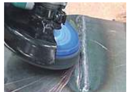
*Removing blue weld discoloration
