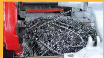
Fig. 1 Chips from cut threads
