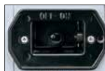
Anti-crash switch: Switch protects die head from touching hand wheel
