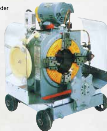
Cutting machine designed for the M No. 6 threading machine. It had 4 bite blades and could cut stainless steel pipes
