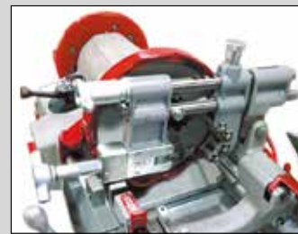
Blade-type cutter on N100A
