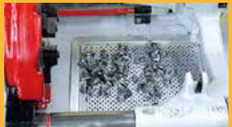
Fig. 2 Chips from roll threads
