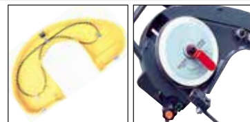
Fig.11 Spare blade can be stored inside the cover.(Extra blade : option)
